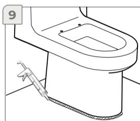
A line drawing of a toilet base. A silicone bead is being applied to the joint between the toilet base and the floor. A small callout box labeled '9' is in the top left corner.
